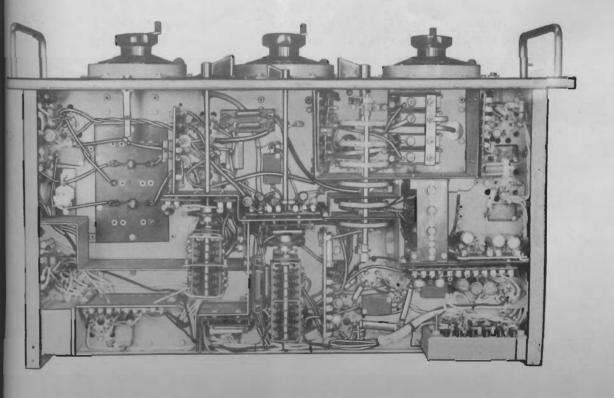
Aerial tuning unit for Transmitter 5AB. Matches the impedence of the transmitter to the impedence of the trunk.
